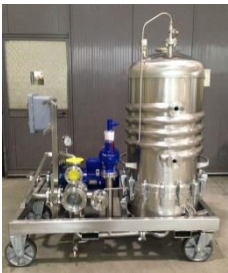
Plate filter with trolley, valves and pump
