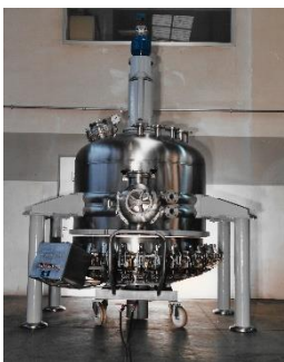
Agitated Nutsche filter with auto-closing system
